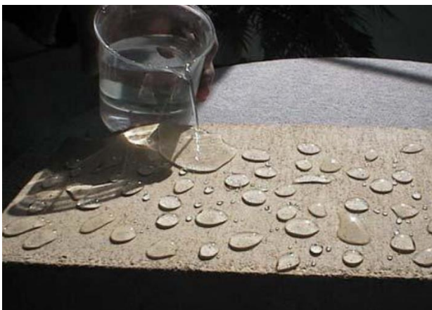
Water repellent effect on a concrete block containing silicone
